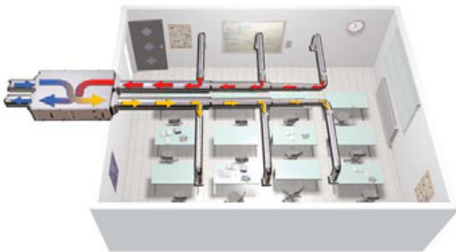
Typical school classroom
