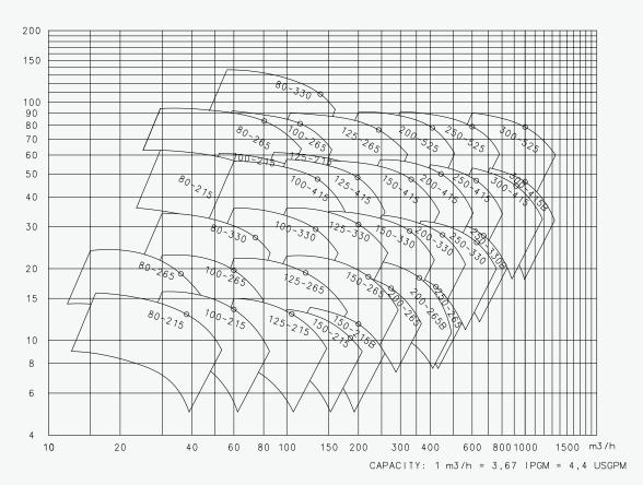
DESMI performance curves and tests of centrifugal pumps are according to EN/ISO 9906 grade 2B as standard - other grades on request
