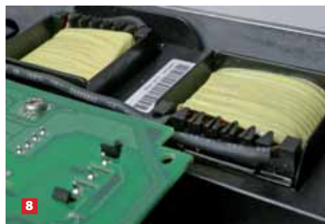
DC coils reduce harmonic noise and protect the drive. Also EMC filters are integrated (meets EN 55011 A2, A1 or B).
